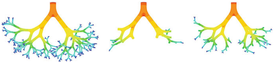
Fig. 63.3 Static pressure contours for the fully resolved eight generation lung airway model ( left ), the 4 path FPE ( middle ), and the 16 path FPE model ( right ) during steady inhalation (higher pressure at inlet, lower pressures at exits)
